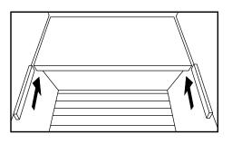
**Optional:** After the bench is installed, you can slide in the included wood pieces to prevent the bench from sliding left to right. One piece can be placed on each side next to the bench. If you decide to flip the reversible bench over, please remove the wood pieces first.
