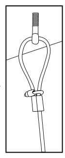
4. Repeat section 3 above with the other end of the metal cable securing it to the J bolt ground anchor. Be sure the cable is pulled tight.
