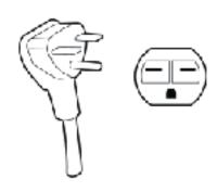
240 V / 15 amps electrical circuit required. NEMA 6-15p
