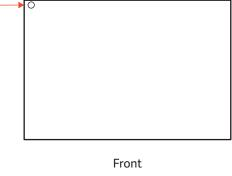
Power cord comes out of the roof of the sauna and is approximately 8 ft long.
