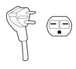
240V / 15 Amp Electrical Circuit Required NEMA 6-15p
