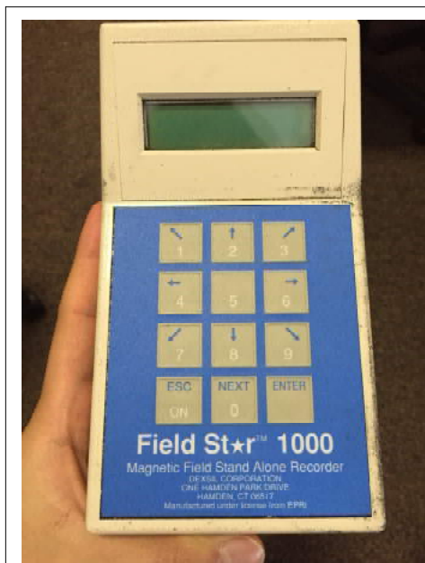
FieldStar 1000 Gaussmeter used during EMF/EMC Study
