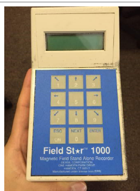
FieldStar 1000 Gaussmeter used during EMF/EMC Study
