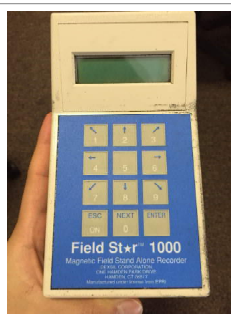
FieldStar 1000 Gaussmeter used during EMF/EMC Study
