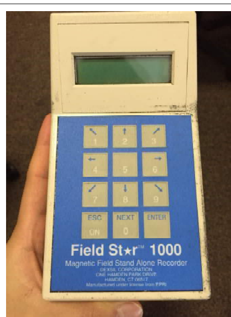
FieldStar 1000 Gaussmeter used during EMF/EMC Study
